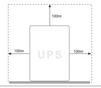
The UPS is intended for indoor use only. Although your UPS is very rugged, its internal components are not sealed from the environment. Kindly note the following. \*Avoid direct sunlight.
